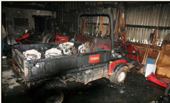
Workman Plastic Melted
